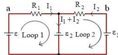
**Figure 6.** Complex circuit with two sources of electric current
