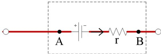
**Figure 4.** A battery and the direction of current in the battery
