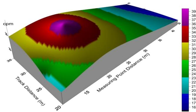
**Figure 1.** Three-dimensional curve of radioisotope count in rock minerals in Oesuu, Central Kupang
