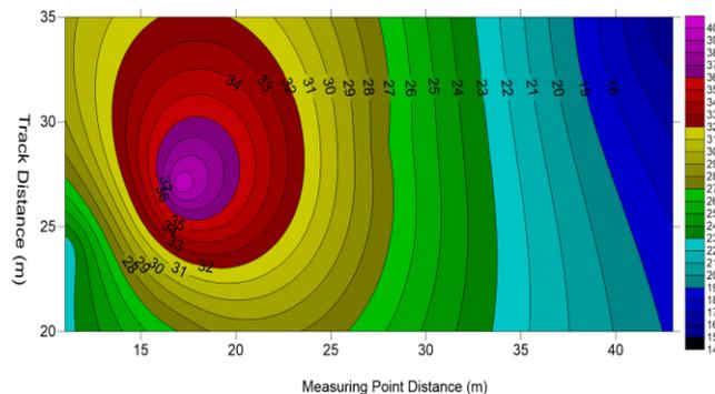
**Figure 3.** Contours of radioisotope count fluctuations in rock minerals in Oesuu, Central Kupang
