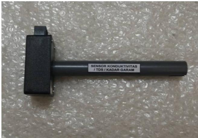
Figure 5. TDS Sensor/Conductivity
