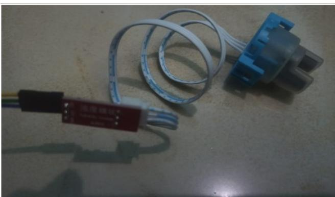
Figure 6. Turbidity Measuring Sensor
