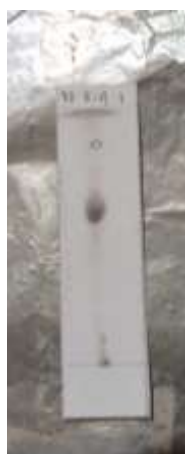
Figure 3. Thin layer chromatography test (n-heksana : etil aasetat, 4 : 1)
