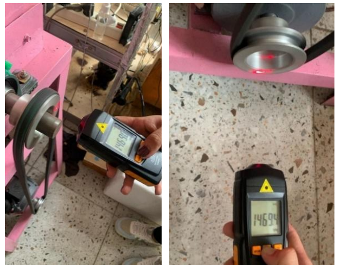
Figure 6. Rotational Speed Measurement of Upper and Lower Pulleys via Tachometer
