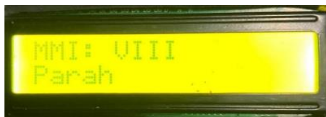
Figure 5. LCD display shows severe MMI VIII scale conditions
