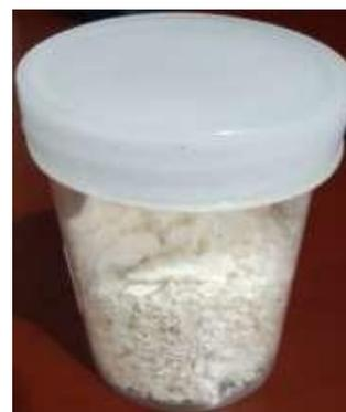
Figure 2. Regenerated cellulose obtained after mercerization
