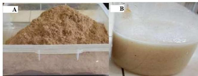
Figure 1. (A) Durian rind powder; (B) Holocellulose
