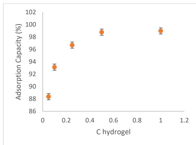
**Figure 5.** Adsorption capacity of durian rind-based hydrogel at varying concentrations of methylene blue
