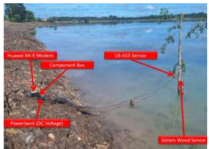
Figure 6. Gelang wood sensor application in monitoring water level height in a lake
