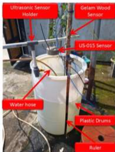
Figure 2. Gelam wood sensor calibration procedure
