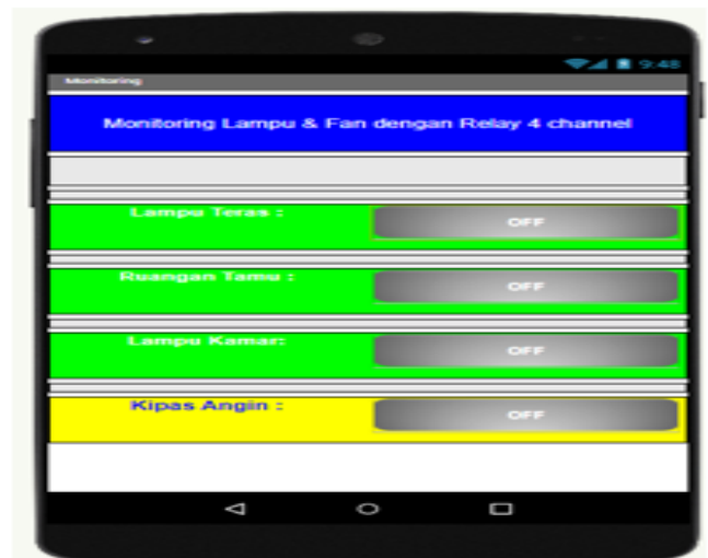
Figure 4. Design of Monitoring Interface for Lights and Fans
