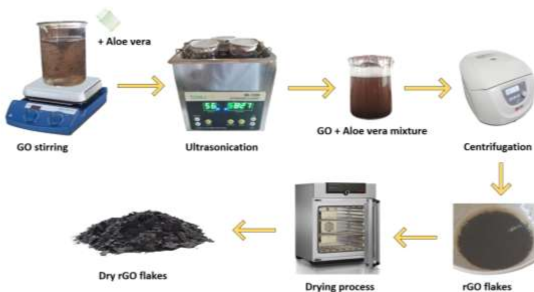
Figure 1. Synthesis stage of rGO using Aloe vera extract
