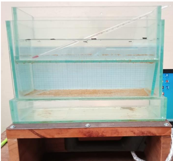
Figure 5. Photo of the RBC observation instrument
