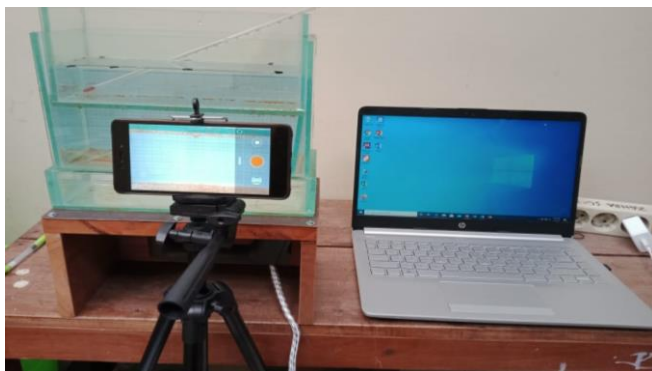
Figure 6. Photo of RBC observation device set up
