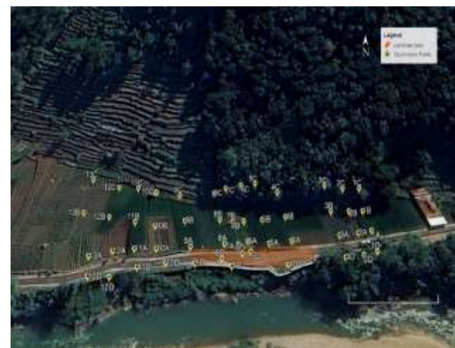
Figure 2. The research site is a subsiding road segment (shown in orange) aligned west-east, adjacent to the river. The allocation of measuring sites is also displayed.
