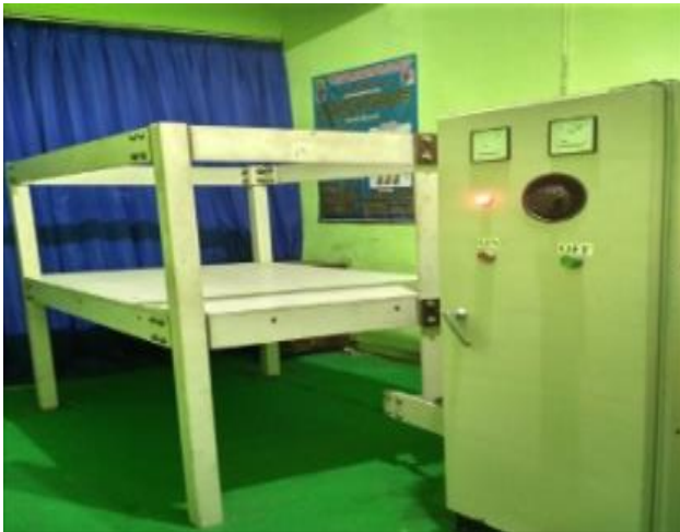
Figure 1. Current Transformer (ELF Electromagnetic Wave Source)
