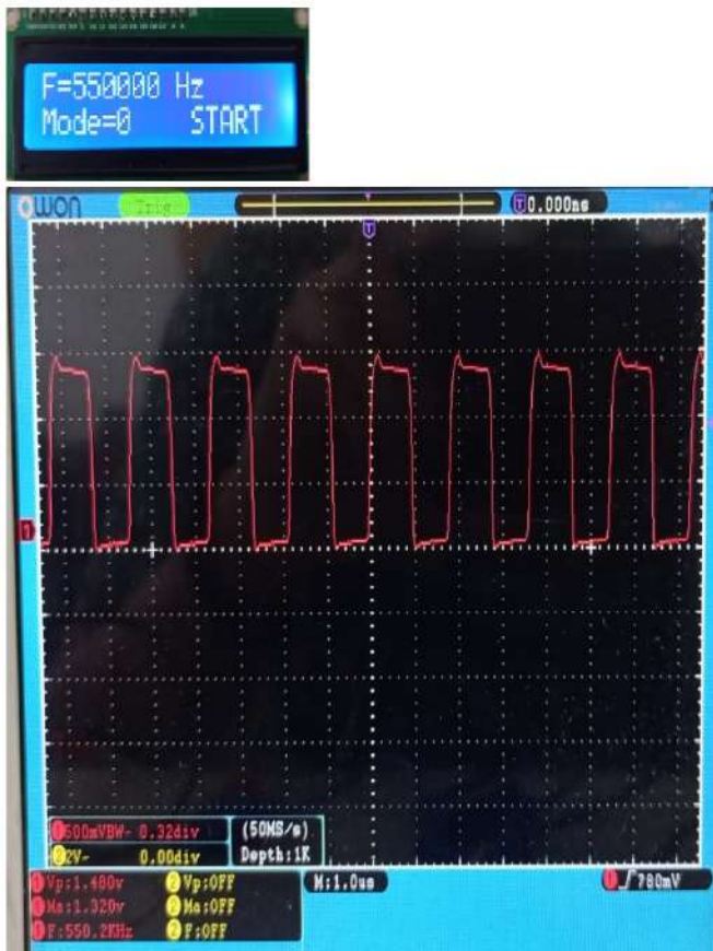
Figure 14. Measurement of TP1 Signal Frequency 550 KHz
