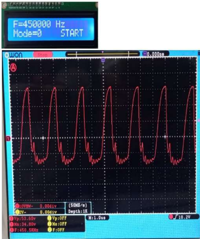
Figure 21. Measurement of TP2 Signal Frequency 450 KHz with beef load
