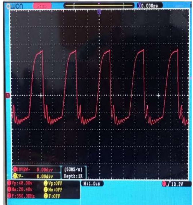
Figure 19. Measurement of TP2 Signal Frequency 350 KHz with beef load
