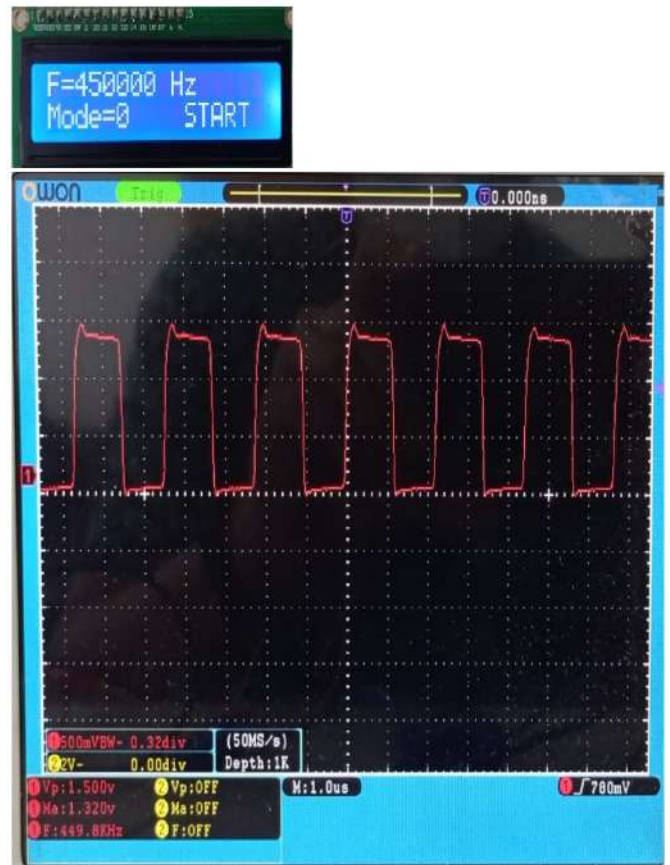
Figure 12. Measurement of TP1 Signal Frequency 450 KHz
