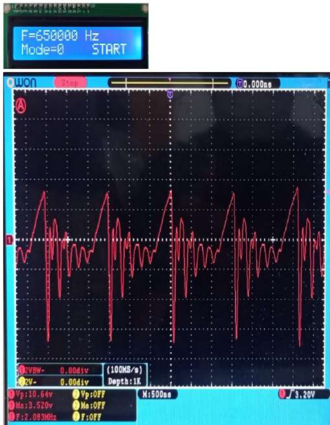
Figure 25. Measurement of TP2 Signal Frequency 650 KHz with beef load
