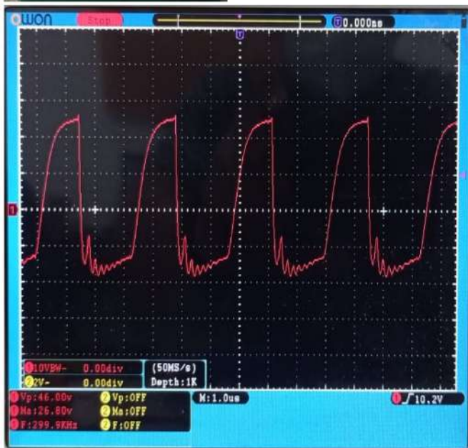
Figure 18. Measurement of TP2 Signal Frequency 300 KHz with beef load
