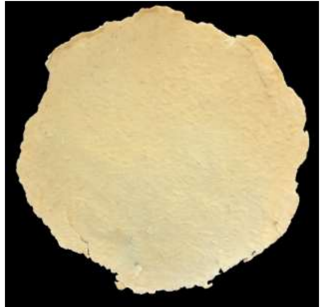
Figure 2. Macroscopic appearance of the fabricated chitosan membrane filter derived from shrimp-shell waste.
