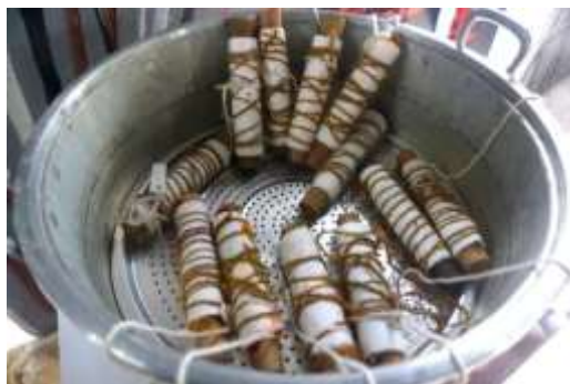
Figure 2. Fixation and steaming process using tunjung
