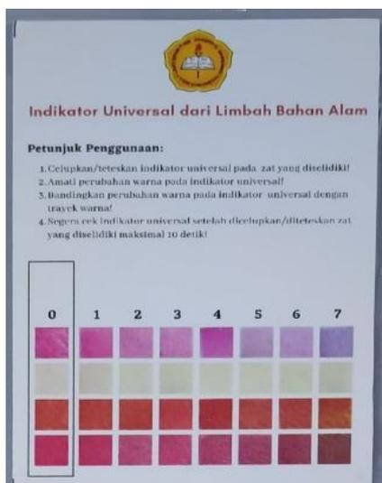
Figure 3. Universal Indicator Box Appearance (front side)
