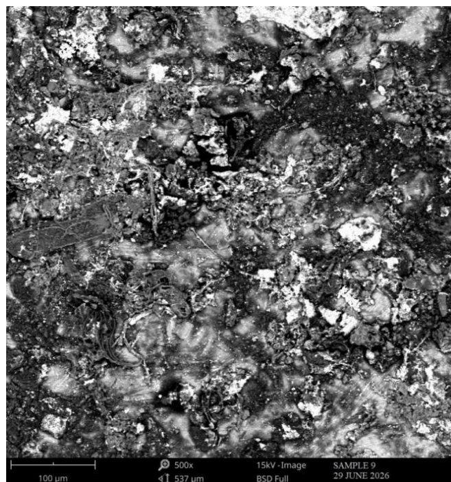
Figure 6. SEM micrograph of C9 (10 wt.% coconut fibre, 10 wt.% corncob ash) (500× magnification, FOV 537 µm, 15 kV, backscattered-electron detector).
