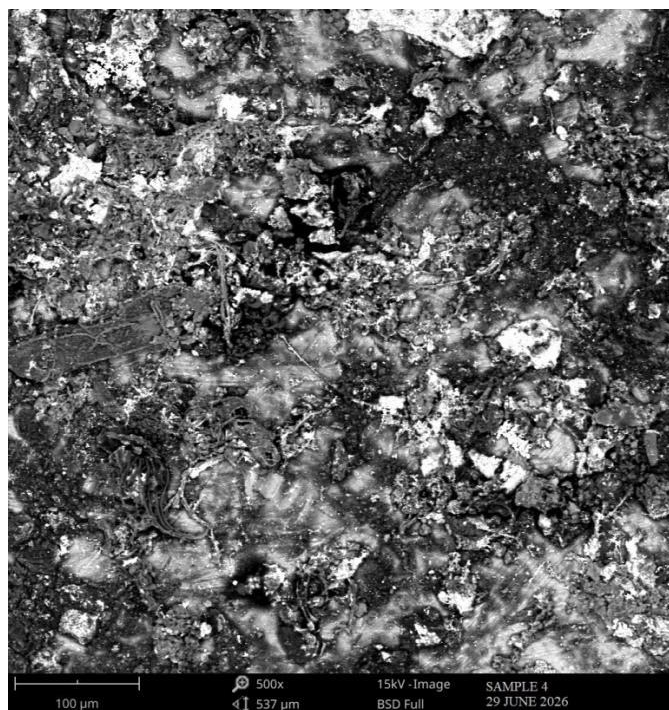
Figure 4. SEM micrograph of C4 (5 wt.% coconut fibre, 3 wt.% corncob ash) (500× magnification, FOV 537 µm, 15 kV, backscattered-electron detector).
