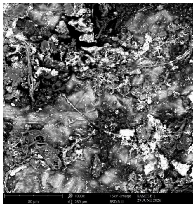
Figure 2. SEM micrograph of C1 (3 wt.% coconut fibre, 3 wt.% corncob ash) (1000× magnification, FOV 269 μm, 15 kV, backscattered-electron detector).
