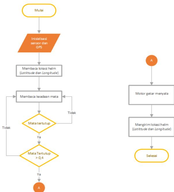
**Figure 2.** Helmet Algorithm Design
