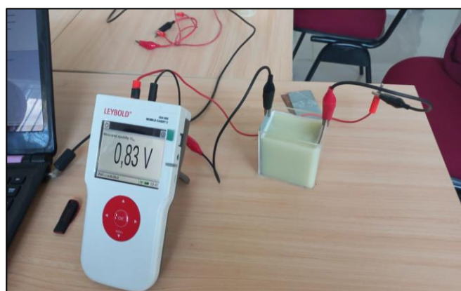
Figure 2. voltage and current measurement in Galvanic cell with concentration of 60%
