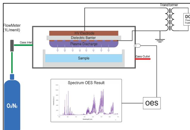
**Figure 1.** Schematic of surface dielectric barrier discharge nonthermal plasma
