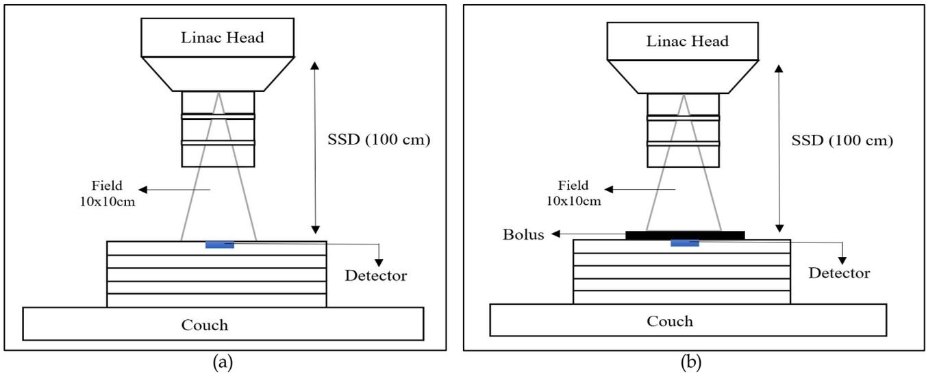
Figure 1. The Set Up of Surface Dose Measurement (a) without bolus (b) with bolus
