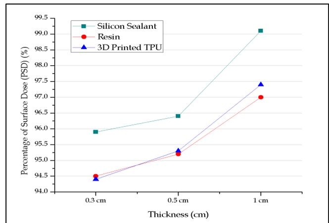
**Figure 3.** Percentage of Surface Dose (PSD) for Some Thickness for Each Sample Bolus on 10 MeV
