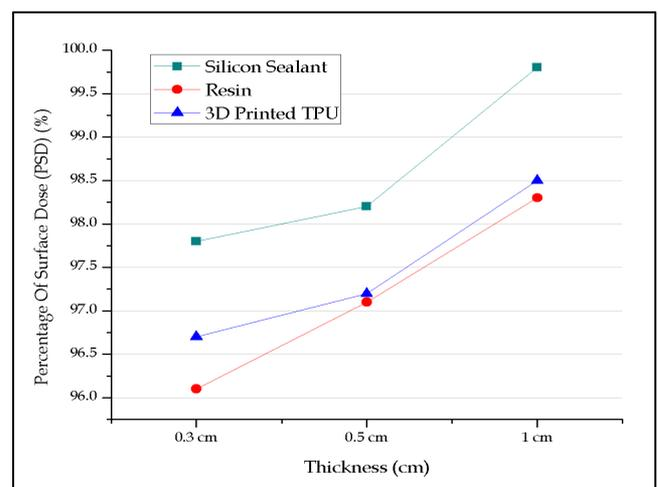
**Figure 4.** Percentage of Surface Dose (PSD) for Some Thickness for Each Sample Bolus on 12 MeV
