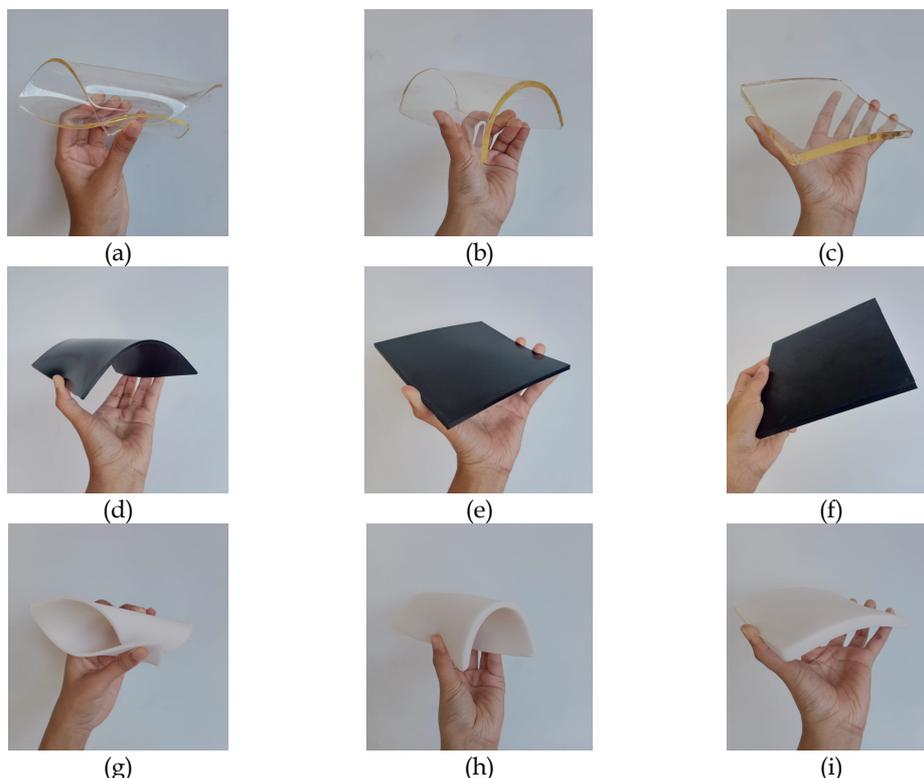
**Figure 2.** Some In-House Bolus samples with 15x15 cm<sup>2</sup> and variations in thickness of (a) 0.3 cm resin (b) 0.5 cm resin (c) 1 cm resin (d) 0.3 cm 3D printed TPU (e) 0.5 3D printed TPU (f) 1 cm 3D printed TPU (g) 0.3 cm silicon sealant (h) 0.5 cm silicon sealant (i) 1 cm silicon sealant.
