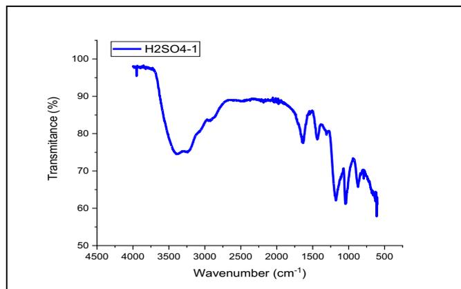
**Figure 8.** FTIR transmittance spectrum pattern of PVA-Enzyme/GA/PPy+H<sub>2</sub>SO<sub>4</sub>/PVC-KTpCIPB-o-NPOE indicator electrode one drop
