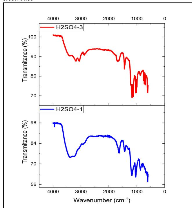
**Figure 7.** FTIR transmittance spectrum pattern of PVA-Enzyme/GA/PPy+H<sub>2</sub>SO<sub>4</sub>/PVC-KTpCIPB-o-NPOE indicator electrode (a) one drop, (b) three drops
