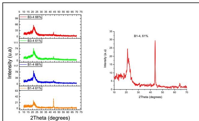
**Figure 5.** XRD Diffraction Spectrum Pattern PVA-Enzyme/GA/PVC-KTpCIPB-o-NPOE indicator electrode
