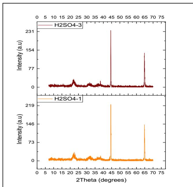
**Figure 6.** XRD Diffraction Spectrum Pattern PVA-Enzyme/GA/PPy+H<sub>2</sub>SO<sub>4</sub>/PVC-KTpCIPB-o-NPOE indicator electrodes
