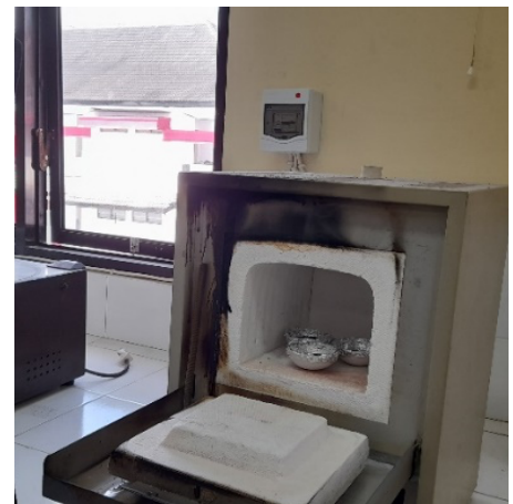
Figure 8. Sample calcination process at 1100°C
