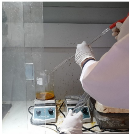
Figure 4. The reaction process for solutions 1 and 2 and dripping with NH 4 OH
