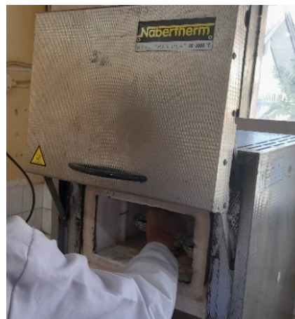
Figure 7. Sample calcination process at 400°C
