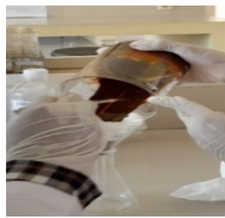
Figure 5. Sample filtering and waiting for the neutralization of the sample until the pH is neutral
