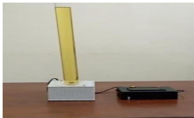
Figure 5. A viscometer educational aid using arduino uno
