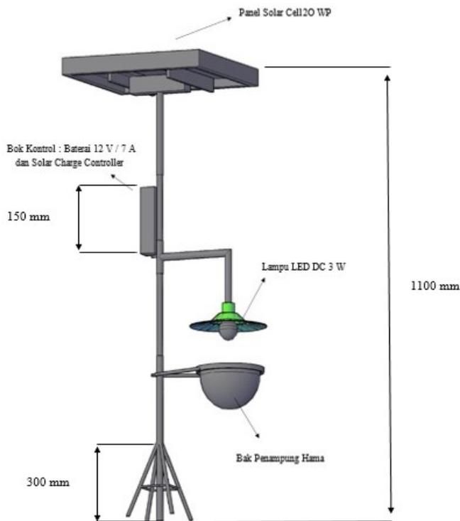
Figure 1. Pest Trap Design
