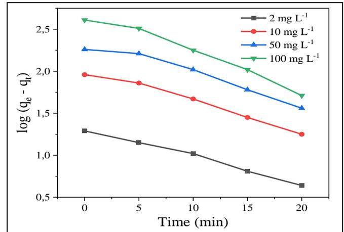
Figure 7. The adsorption of MG onto RGO follow first-order kinetics
