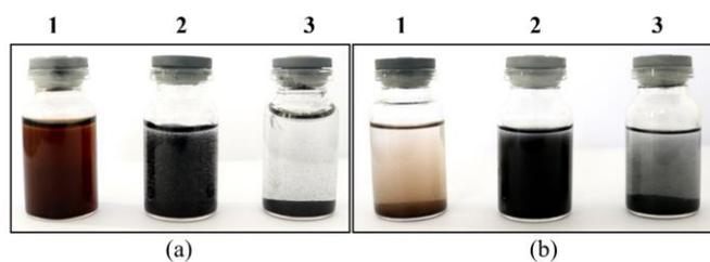
Figure 4. Dissolving samples sequentially, namely (1) GO, (2) RGO and (3) graphite in a) water and b) ethanol
