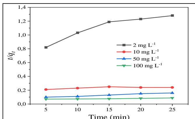
Figure 8. The adsorption of MG onto RGO follow second-order kinetics
