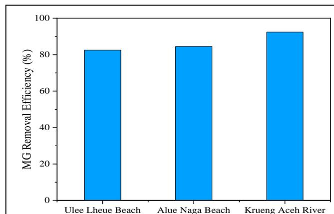
**Figure 8.** MG Removal efficiency with RGO from a real water sample.
