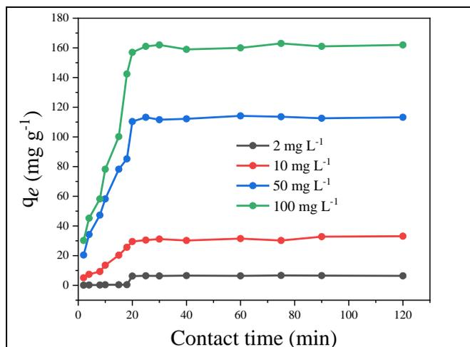
Figure 5. The influence of contact time and initial MG concentration on the adsorption capacity of RGO
