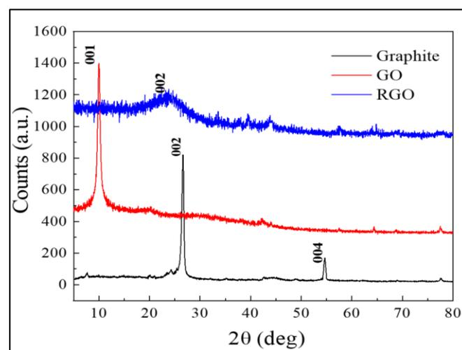
Figure 2. X-ray diffraction patterns on graphite, GO, and RGO samples
