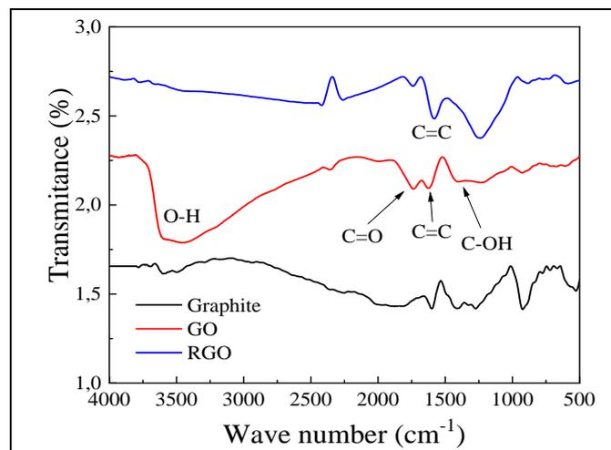
Figure 3. FTIR spectra of graphite, GO, and RGO samples
