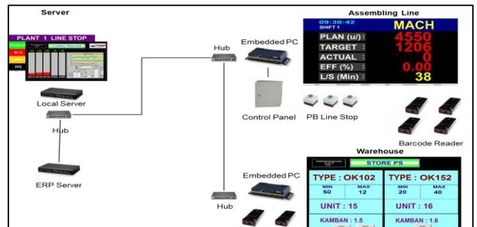
Figure 1. Design of Warehouse Control Tower (WCT) System
