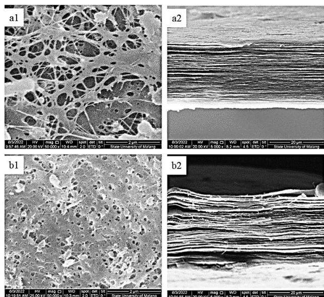
**Figure 4.** SEM image: a1. BC (50000 $\times$ ); a2. cross section of BC (50000 $\times$ ); b1. BC/ $\text{Al}_2\text{O}_3$  composite (50000 $\times$ ); b2) Cross section of the BC/ $\text{Al}_2\text{O}_3$  composite (5000 $\times$ ).
