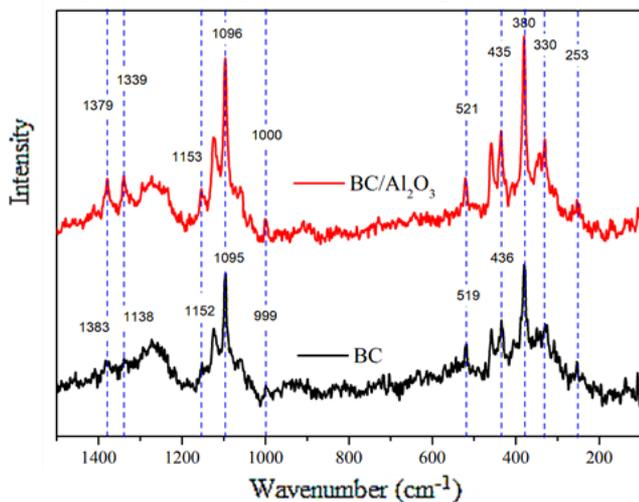
**Figure 3.** Spectral comparison Raman BC and BC/ $\text{Al}_2\text{O}_3$  composites
