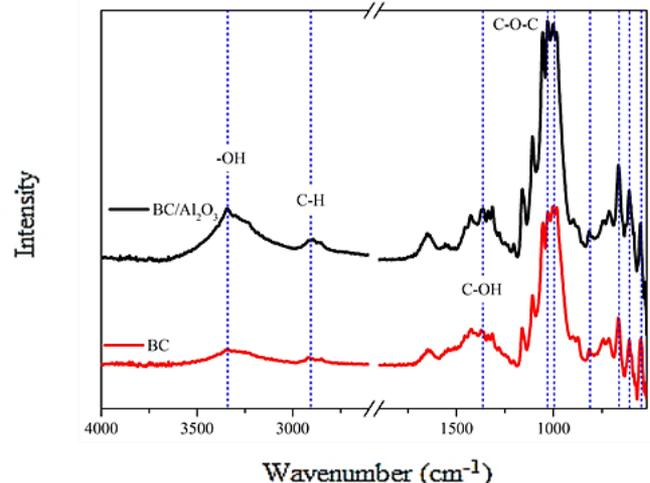
**Figure 2.** FTIR-ATR BC and BC/Al<sub>2</sub>O<sub>3</sub> composite
