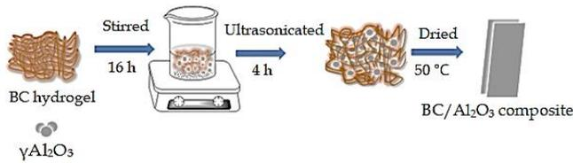
**Figure 1.** The schematic representation of a ex situ method to synthesize BC/Al<sub>2</sub>O<sub>3</sub> composite
