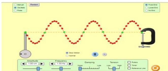
Figure 2. Tied end stationary waves
