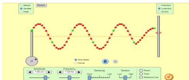
Figure 3. Free end stationary waves
