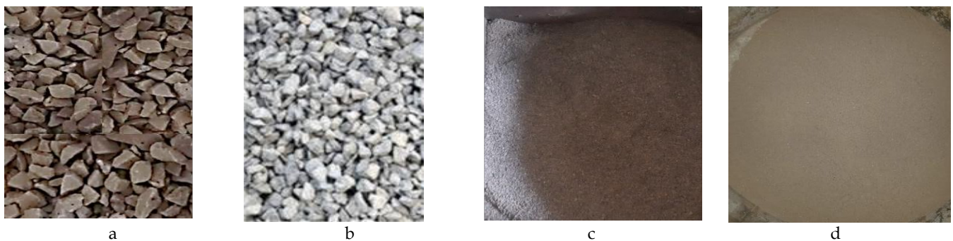
Figure 1. (a) Artificial Coarse Aggregate, (b) Natural Coarse Aggregate, (c) Fine Aggregate and (d) Filler
