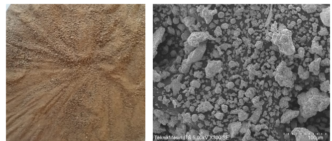
Figure 3. PLTU Jeranjang fly ash and morphology based on SEM tests
