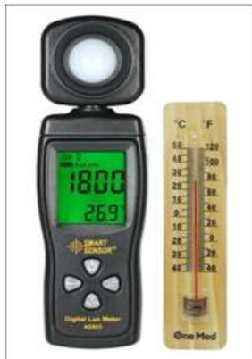
Figure 1. Lux meter and room thermometer
