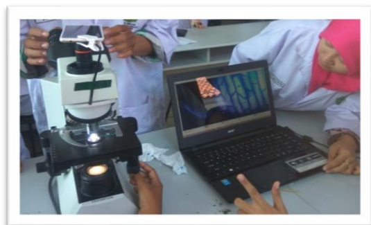
Figure 2. Modification of Light Microscope into Digital Microscope
