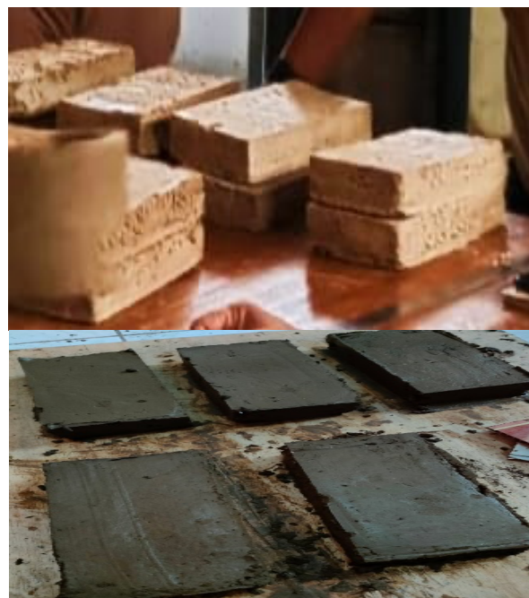
Figure 1. Display of brick products without burning
