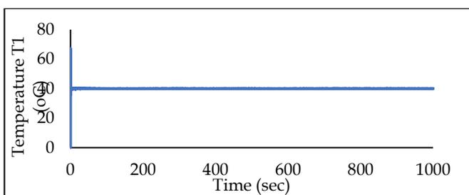
Figure 9. PID controller simulation results with the addition of decoupling at temperature  $T_1$
