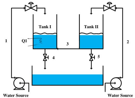
**Figure 2.** Coupled tank system scheme
