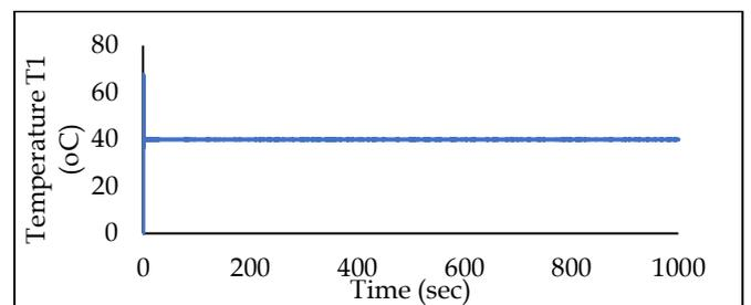
**Figure 6.** PID controller simulation results without the addition of decoupling at temperature  $T_1$
