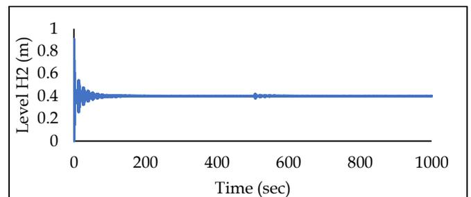
**Figure 5.** PID controller simulation results without the addition of decoupling at level  $H_2$
