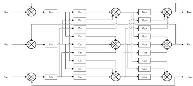
**Figure 3.** Closedloop MIMO 3×3 simulation with decoupling
