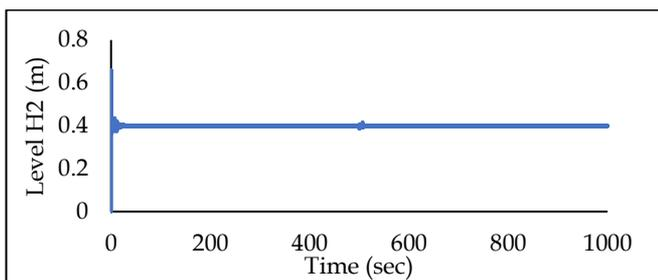
Figure 8. PID controller simulation results with the addition of decoupling at temperature  $H_2$
