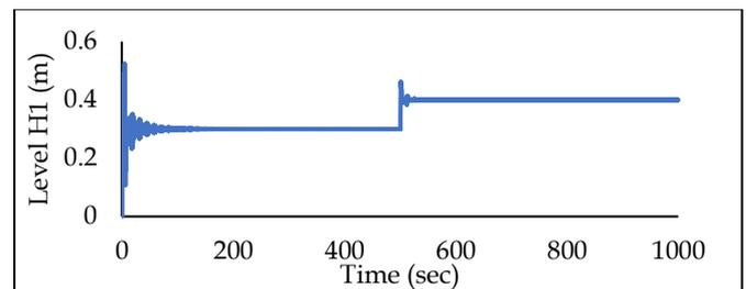
**Figure 4.** PID controller simulation results without the addition of decoupling at level  $H_1$
