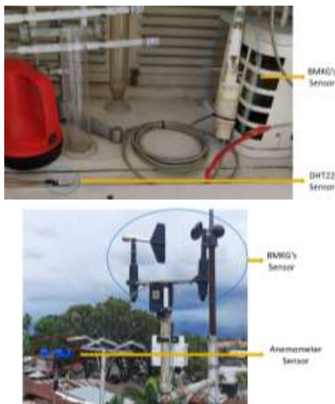
Figure 4. Installation of prototype sensors at BMKG
