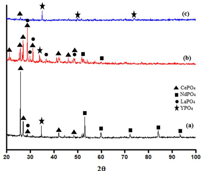
**Figure 4.** The XRD pattern of (a) natural monazite from Bangka, (b) product from mechanical-magnetic separation, & (c) impurities from mechanical-magnetic separation.
