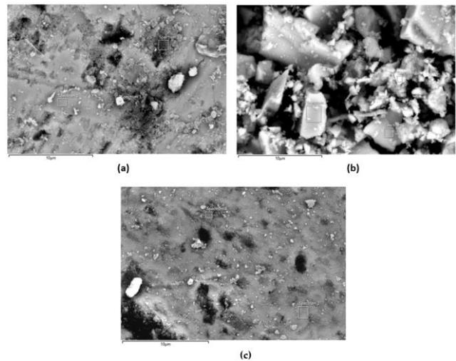
**Figure 3.** The element distribution on the morphology of: (a) natural monazite from Bangka; (b) product from mechanical-magnetic separation; and (c) impurities from mechanical-magnetic separation.
