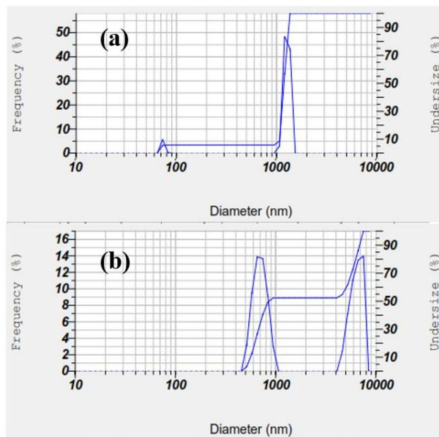
**Figure 5.** The distribution of particle diameters sieved 325 mesh from mechanical-magnetic separation: (a) product, and (b) impurities. (Note: Qualitatively original measurements; quantitative data was not provided at the time of measurement.)
