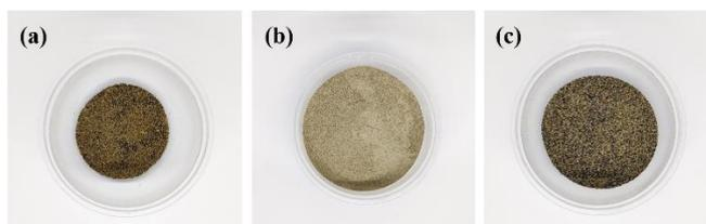
Figure 2. Photo of the physical appearance of monazite before and after the purification process: (a) natural monazite from Bangka [MZ #1], (b) product from mechanical-magnetical separation [MZ #2], and (c) impurities from mechanical-magnetical separation [MZ #3].
