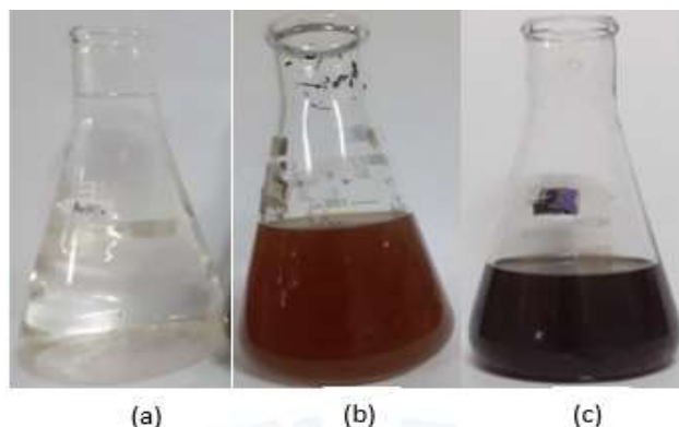
Figure 1: AgNO 3 solution (a), SPE (b), AgNPs solution produced (c).
