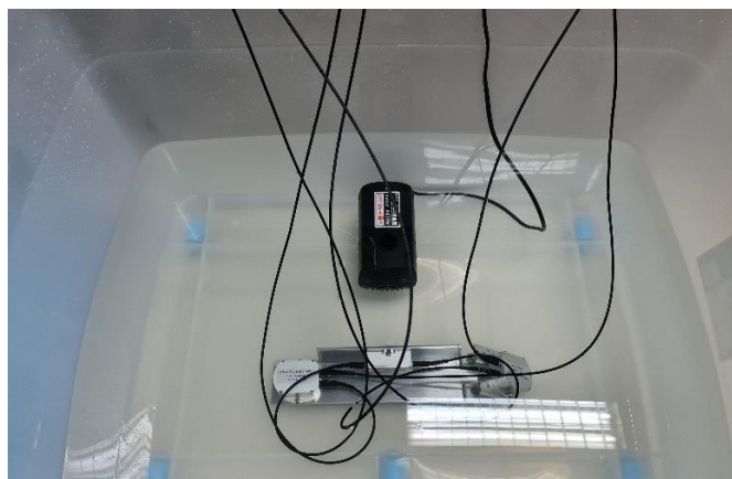
Figure 5. Vibration source at 10 cm from FBG Y
