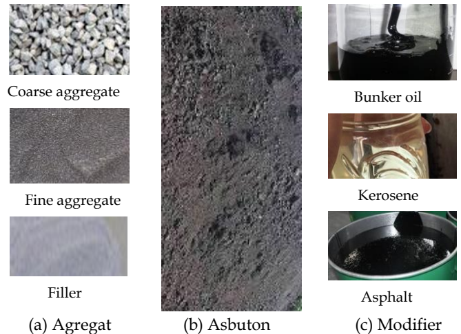
Figure 1. Asphalt mixture material
