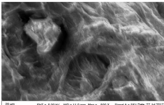
Figure 4. SEM micrograph of cocoa pod shell charcoal
