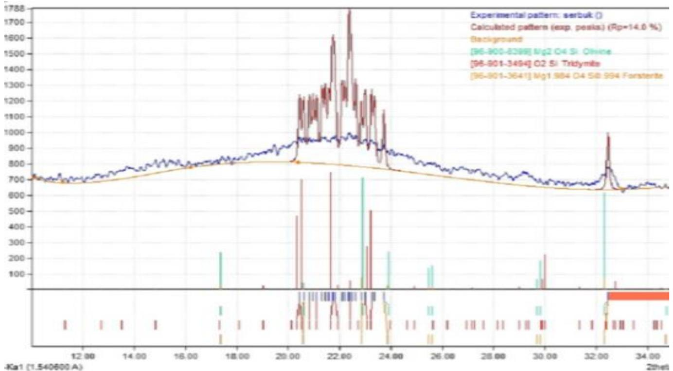
Figure 5. XRD diffractogram pattern of cocoa pod shell charcoal
