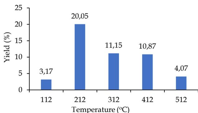
**Figure 1.** The effect of temperature on the yield of liquid smoke from cocoa pod skin
