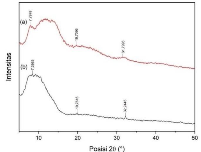
**Figure 6.** X-ray diffractogram (a) of raw material collagen (b) of optimized collagen
