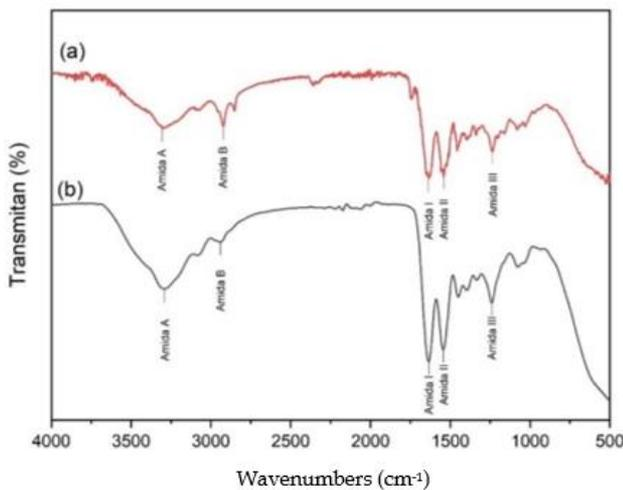
**Figure 3.** Spectrum (a) of raw material collagen (b) of optimized collagen
