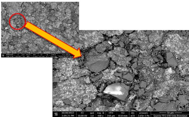
Figure 10. Pressurisation 4500 Psi, sintering 600 °C and sintering holding time 20 min.
