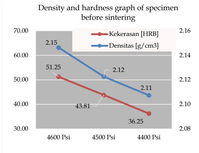
Figure 6. Graph of density and hardness of specimen's before sintering.
