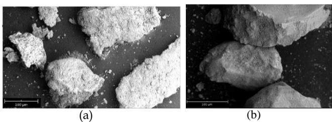
**Figure 1.** Scanning Electron Microscope image of powder (a) Matrix powder (b) SiO<sub>2</sub> reinforcement powder
