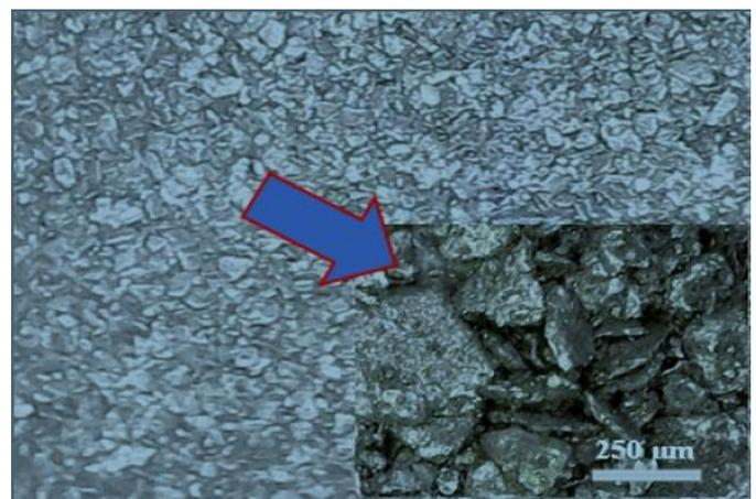
**Figure 3.** Microphoto image of powder resulting from mechanical alloying for 4 hours.
