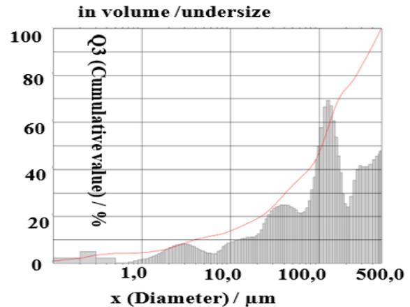
**Figure 2.** Particle Size Analyser Distribution Chart of the 4-Hour Mechanically-Fused Powder
