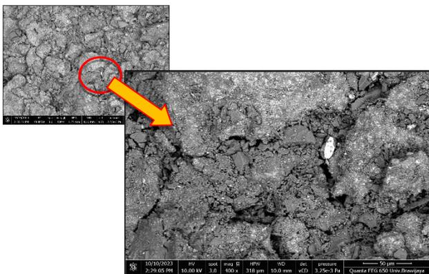
Figure 11. Pressurisation 4600 Psi, sintering 600 °C and sintering holding time 30 min.
