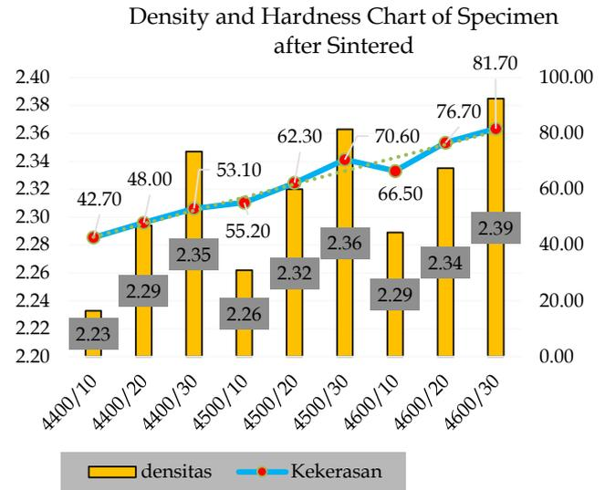
Figure 7. Density and Hardness Graph of Specimens after Sintered
