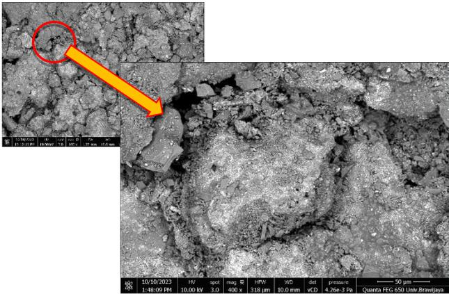
Figure 9. Pressurisation 4400 Psi, sintering 600 °C and sintering holding time 10 min.
