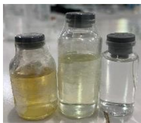
Figure 1. Results of Fractionation of Bitter Melons Extract ( M. charantia ) with Column Chromatography
