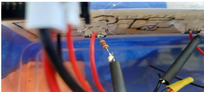
Figure 19. shows the addition of a resistor to one of the legs of the LED light.
